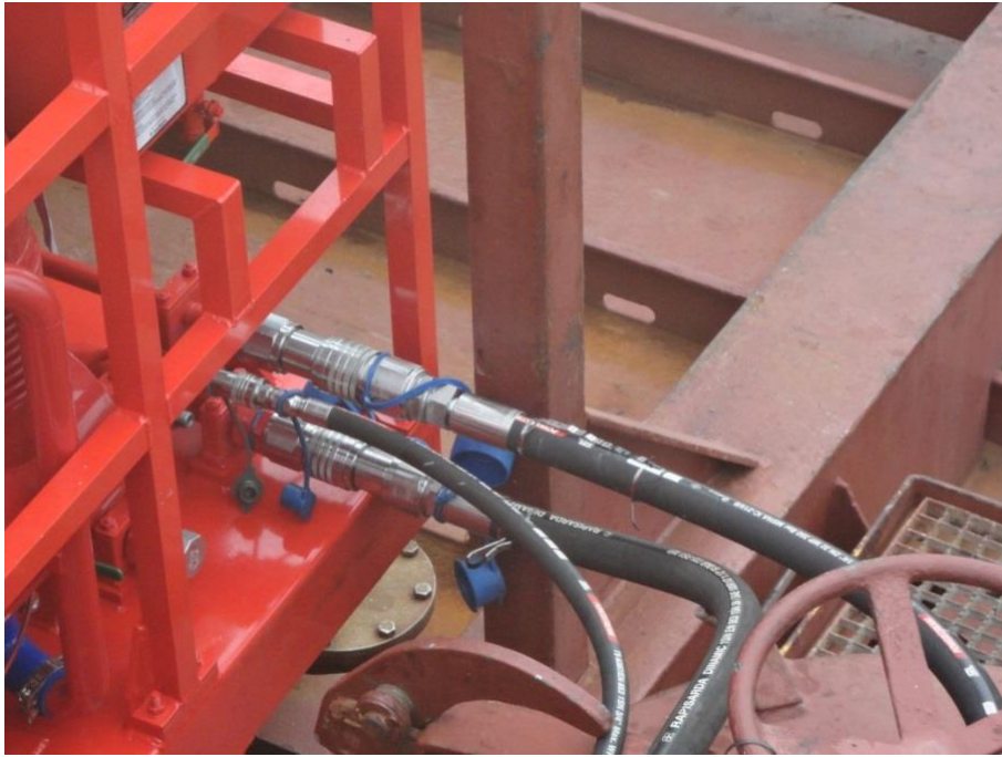
Figure 34. Hydraulic hoses set connected to NorMar DHHP
