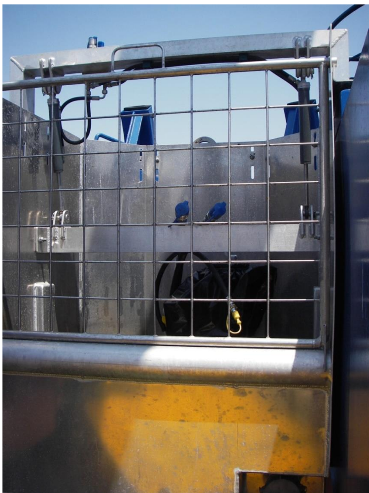
Figure 2. LAMOR Stiff Sweeping Arm LSS 15m – weir skimmer module
