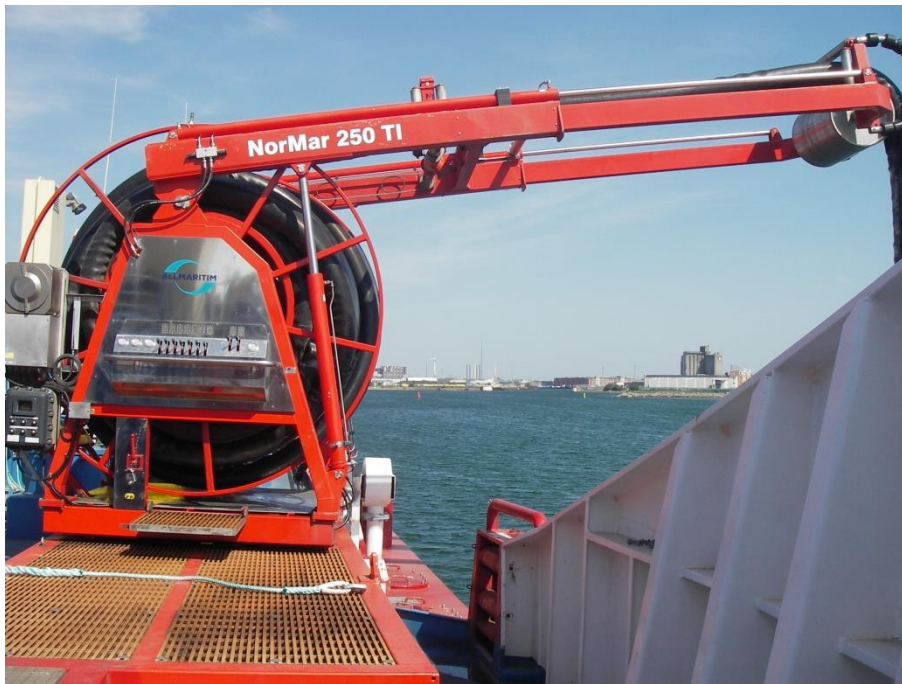
Figure 31. Hydraulically driven reel with 360° turntable, umbilical hose and integrated crane
