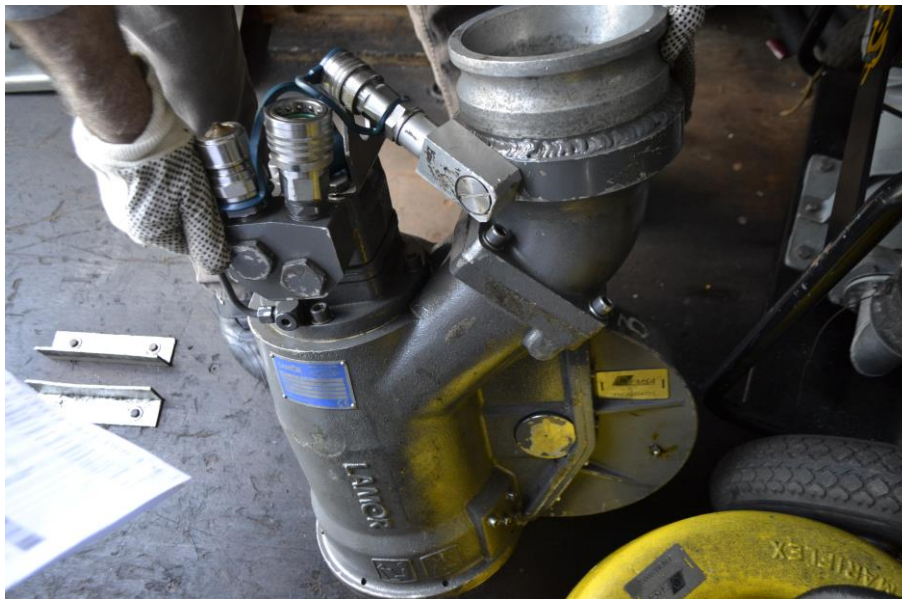
Figure 9. Oil Transfer PDAS Pump Lamor GTA 140
