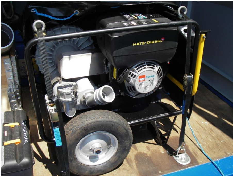
Figure 17. Power pack LPP 14 L with air blower
