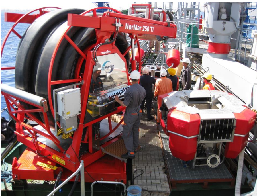
Figure 27. NorMar 250 TI High Capacity Skimmer Set. Brush/disc skimmer head.
