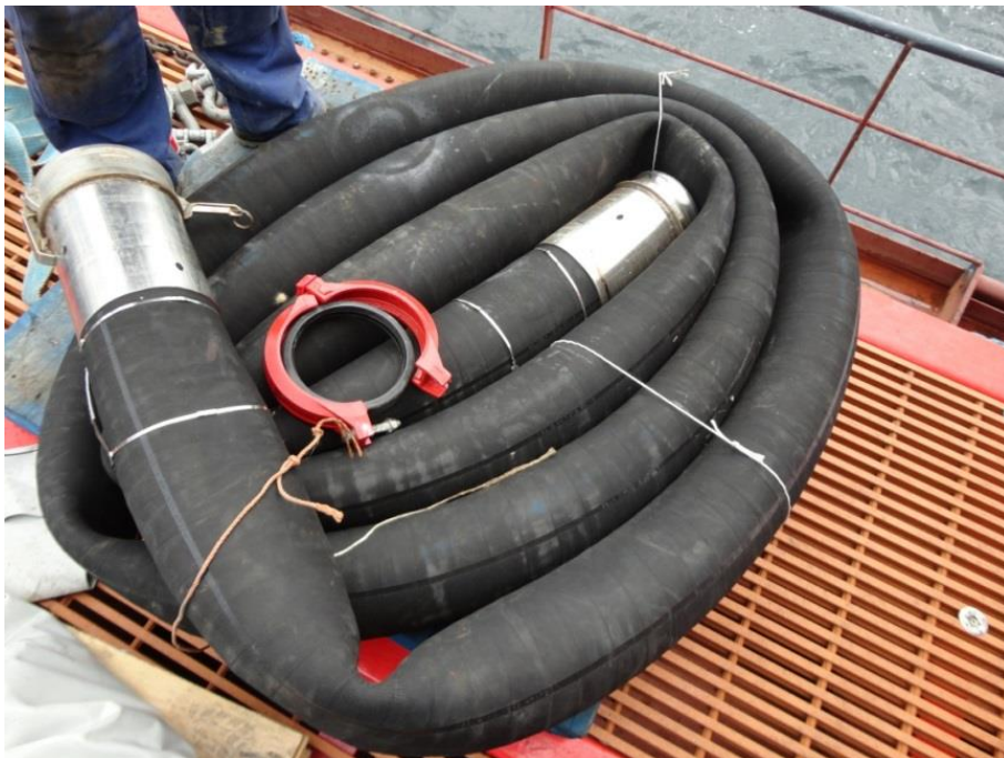
Figure 35. Semi rigid 6" oil hose
