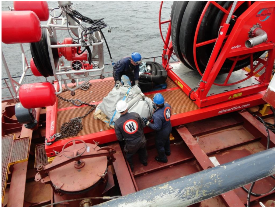
Figure 32. Storage Flat rack 20' with the skimmer system
