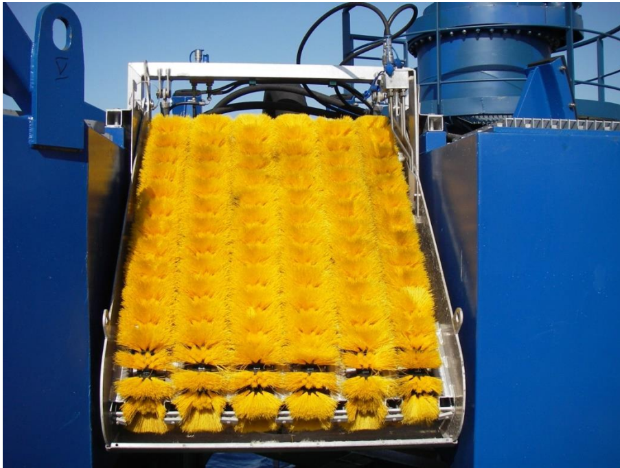
Figure 7. LAMOR Stiff Sweeping Arm LSS 15m – brush skimmer module
