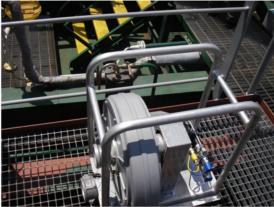
Figure 18. Hydraulic air blower HAB 200
