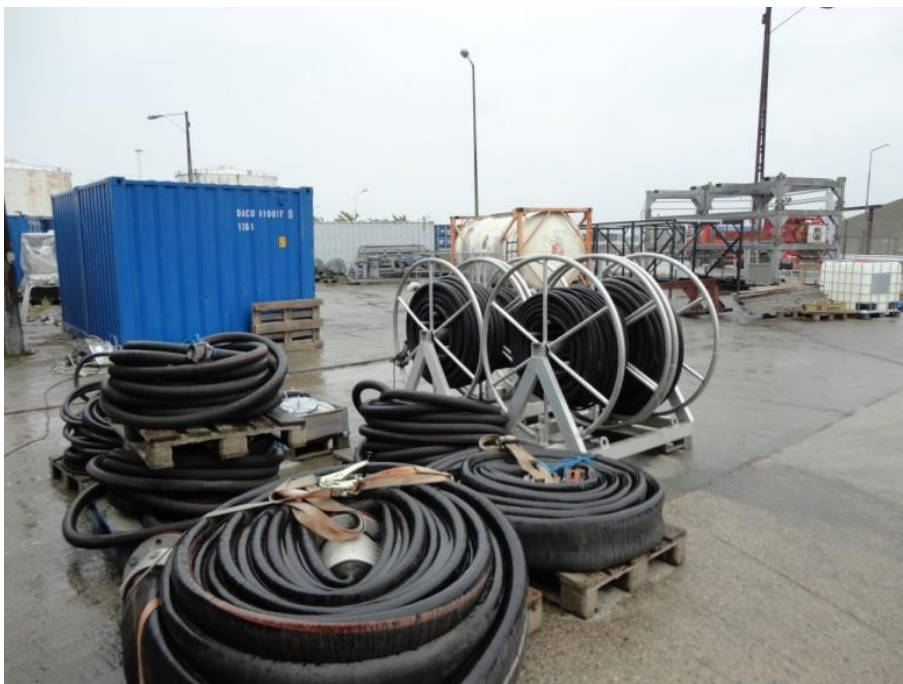
Figure 8. 2 Hose Winders LHW 40/2-AL with hydraulic hoses for LSS 15m
