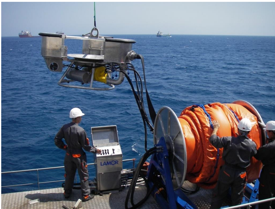
Figure 24. Skimmer Control Panel, 4 valves
