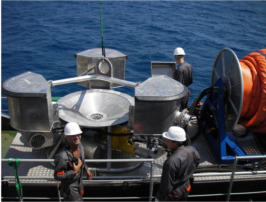
Figure 20. Weir Skimmer LWS 1300 Mk II
