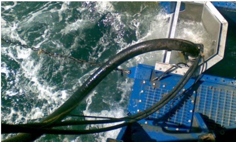
Figure 5. LSS 15 m, oil hose connected to weir skimmer module
